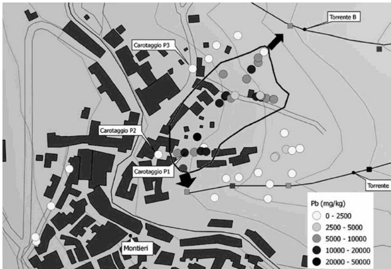
FIG. 8. THE CONCENTRATION OF LEAD IN SOIL SLAG HEAP. THE POLYGON REPRESENT THE WASTE AREA.
