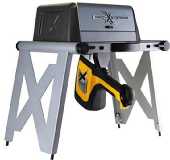
Figure 2. pXRF laboratory station.
