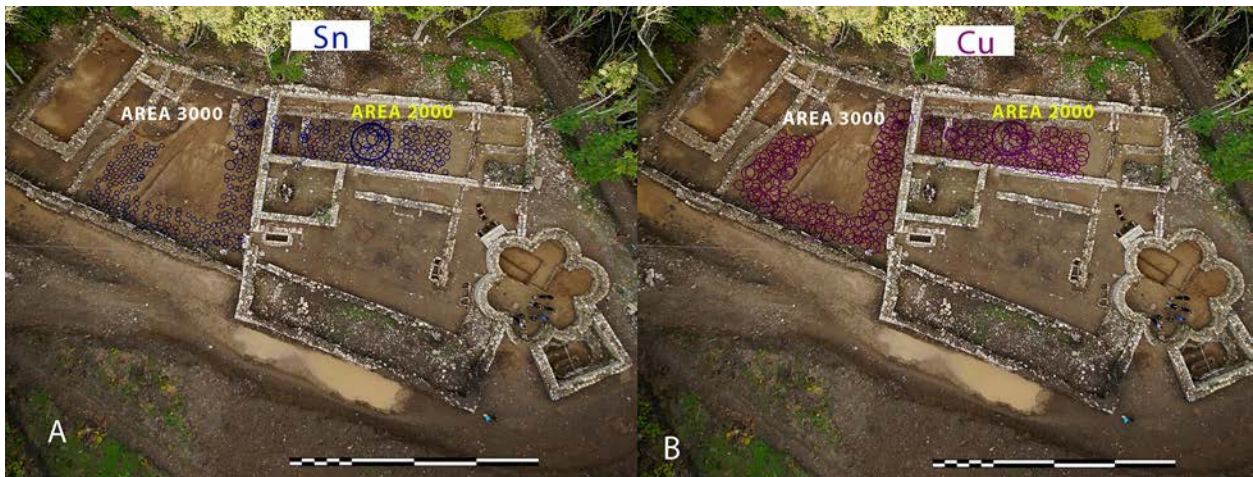
Figure 6. Results of intra-situ pXRF analyses. The ring circumference is proportional to the concentration of the considered chemical element. Analyses have highlighted high concentrations of Sn (A) and Cu (B) on the centre of the area 2000.
